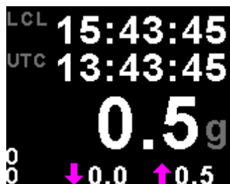
Slip Indicator & OAT disabled, Flight Timer set for remote start/stop
